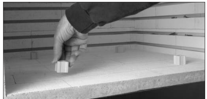
1" (25 mm) posts may give better heat circulation than 1/2" (12.5 mm) posts, depending on the size of your kiln.
