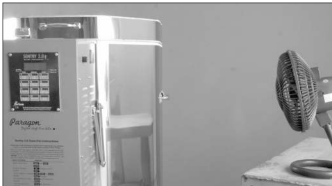
If necessary during hot weather, use a fan to move the heat away from the kiln's switch box.
