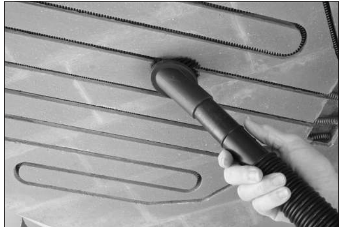
Vacuuming the lid grooves.
