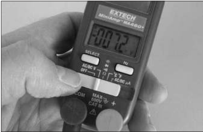
Set a multimeter to Volts AC. See your meter's instruction manual.
