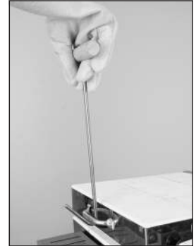
Crash cool by lifting the lid with a Lid Lifter.
