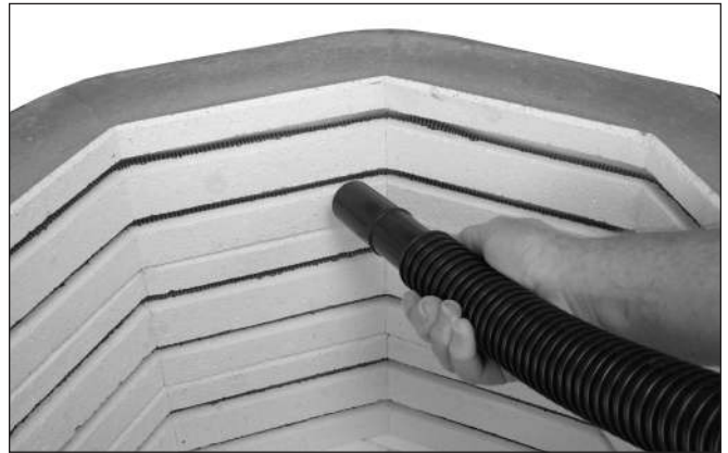
Vacuuming the sidewall grooves.
