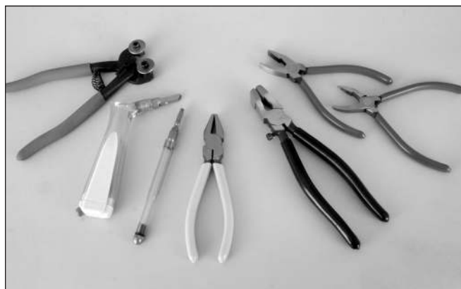
Left to right: nippers, pistol-grip cutter, straight cutter, breaking pliers, running pliers, and two sizes of grozing pliers
