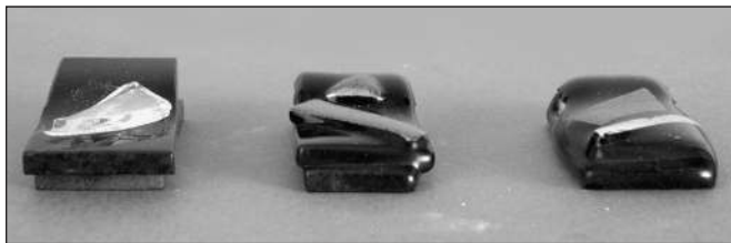
Left to right: tack fuse, medium fuse, and full fuse
