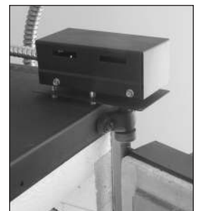
The door safety switch is optional on some kiln models.
