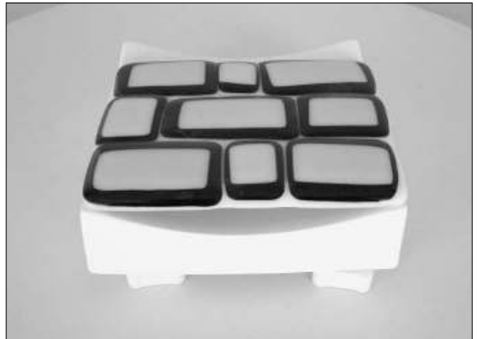
Separate a sagging mold and kiln shelf with ½" (12.5 mm) high posts.
