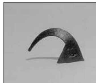
A self-supporting cone fired to maturity. Do not be concerned if the tip is slightly higher or lower than shown.
